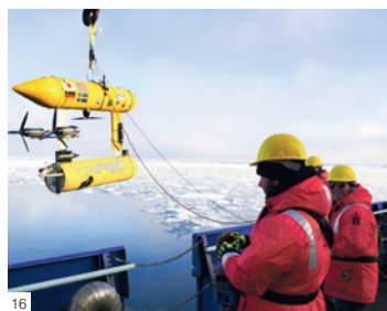
16: An ROV being deployed to survey the underside of Antarctic sea-ice.
