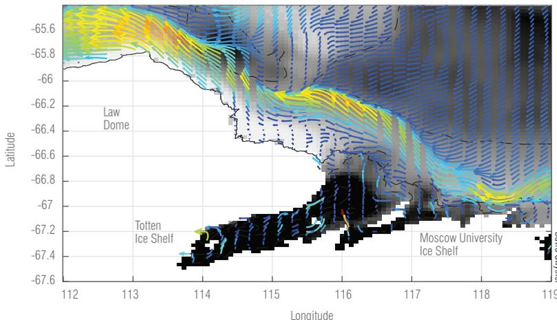
**FIGURE 7:** Map view of the Totten Glacier, showing simulated ocean currents flow westwards past the ice shelf cavity mouth.
