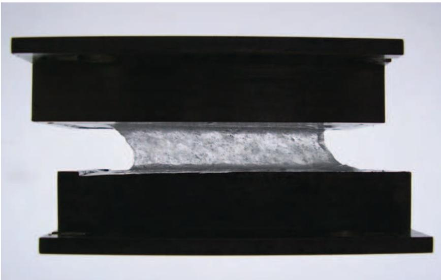
A sample of ice, about 10cm long, that has been deformed in a laboratory experiment to measure its flow rate. In this experiment the lower sample holder was held stationary while the upper holder was forced to the left. The sample was initially rectangular and stretching of the sample due to the very slow deformation of the ice is clearly visible. Experiments like this are important for understanding the physics describing the dynamics of ice flow, such as in the Antarctic Ice Sheet.
