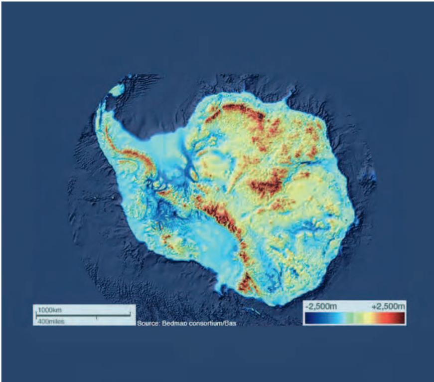
A topographic and bathymetric map of Antarctica without its ice sheets, showing areas grounded below sea level.
